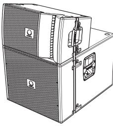
TBV123 ground stack with a TBV118L subwoofer
