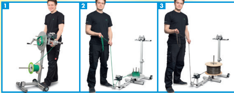
Fig. 1: Winding off the reel onto a ring – ideal for cable fabrication, shipping, or in-store sales. The winding-Ø can be adjusted from 150 to 270 mm/ 5.9" to 10.6". The meter counter* is not included, but is available as an option.
