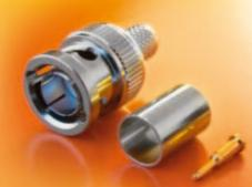
The **BNC** connector (Bayonet Neill Concelman) is one of the best known coaxial plug types and was invented in the late 1940s. It is available with a wave impedance of either 50 or 75  $\Omega$  and is mainly used in radio and video technology, medical engineering and computer technology. Our connectors meet the specifications according to IEC 169-8, MIL-C-39012.
