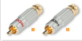
RCA/phono plug, 2-pole. Genuine gold-plated solid pin. Metal housing, Velvet chrome; collet lock fixture. Cable Ø 6.0 - 8.0 mm.
