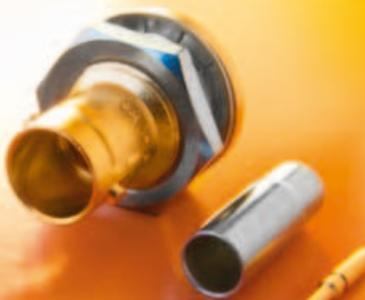
The **BNC** connector (Bayonet Neill Concelman) is one of the best known coaxial plug types and was invented in the late 1940s. It is available with a wave impedance of either 50 or 75 Ω and is mainly used in radio and video technology, medical engineering and computer technology. Our connectors meet the specifications according to IEC 169-8, MIL-C-39012.
