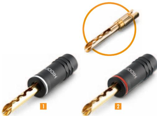
The no-fuss clamping strain relief of the **HICON HI-BM13** ensures negligible contact resistances. The crimping can be done with any common grip wrench, while ideal conductivity is achieved by using BNC/ RG crimping pliers. The banana connector HI-BM13 consists of a screw-on housing and a tight lamella contact.
