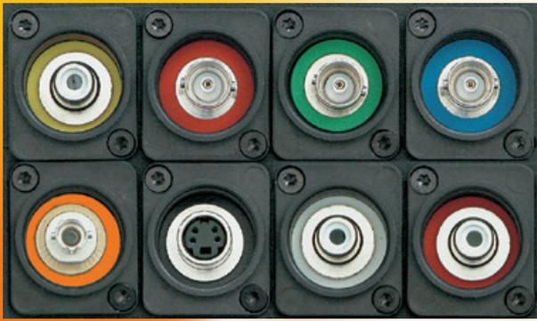
All **HICON** products labelled with the **SYSBOXX** logo can be mounted into the recessed D flange HI-DET or HI-DET-M (Metal version with M3 thread) and will therefore fit into our modular **SYSBOXX** system box (see the "Multicore & Power Distribution Systems" section). The hole diameter of 12.5 mm / 0.5" takes all audio, video, FOC and DATA panel-mount connectors with 1/2" outside thread. For this we recommend our mounting tool WSW16.
