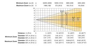
Diameter 10%-50%: beam diameter for 10% and 50% of maximum illumination
