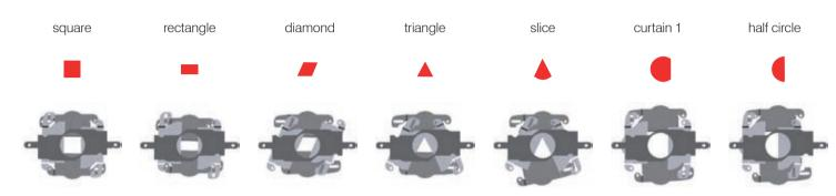
The precision micromechanics of the framing system uses worm gears that ensure perfect repeatability and do away with continuous manual adjustments.
