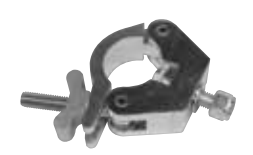
CTC-50HCN • Load Capacity: 750 kg • Captive M12 bolt • T-handle • Narrow Profile • Fits: 50 mm tube • Weight: 0.5 kg • Certifications: TUV
