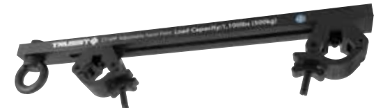
CT-APP CT-APP allows you to create a hang point on the upper chords of box truss to support video walls. The clamp mounting points are adjustable to work with box truss up to 20.5" wide. The Adjustable Panel Point for Video provides a safe and secure connection and supports weights of up to 500 kg.
