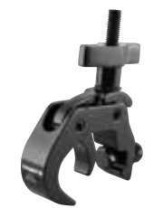
CTC-50G • Load Capacity: 250 kg • T-handle • Fits: 50 mm tube • Weight: 0.45 kg • Certifications: TUV
