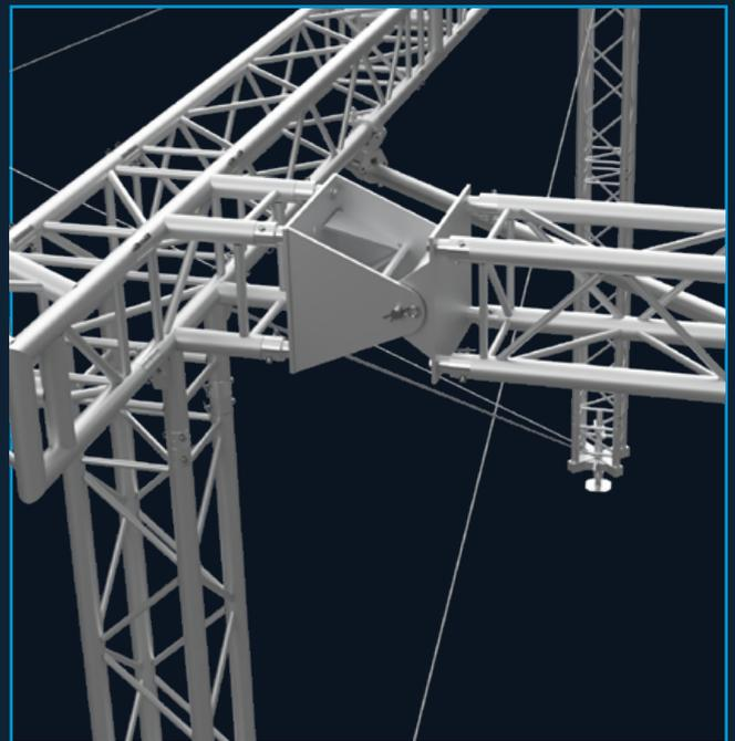
To connect the PA wings to the ARC30 roof, a different corner must be used at the front legs. In addition, a swivel piece must be added to distribute the forces correctly.
