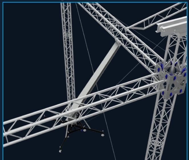
To give horizontal support to the PA-Wings NEXT chooses to use small "H" steel profiles as diagonal support for the PA-Wings. The beams are small and will therefore need small "holes" in the side walls, the other advantage and main reason is the additional pick-point for the PA cluster.
