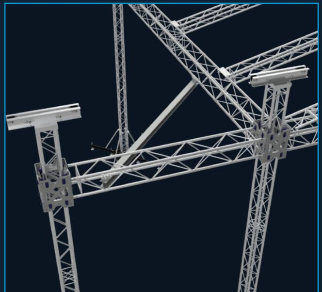
To give horizontal support to the PA-Wings NEXT chooses to use small "H" steel profiles as diagonal support for the PA-Wings. The beams are small and will therefore need small "holes" in the side walls, the other advantage and main reason is the additional pick-point for the PA cluster.
