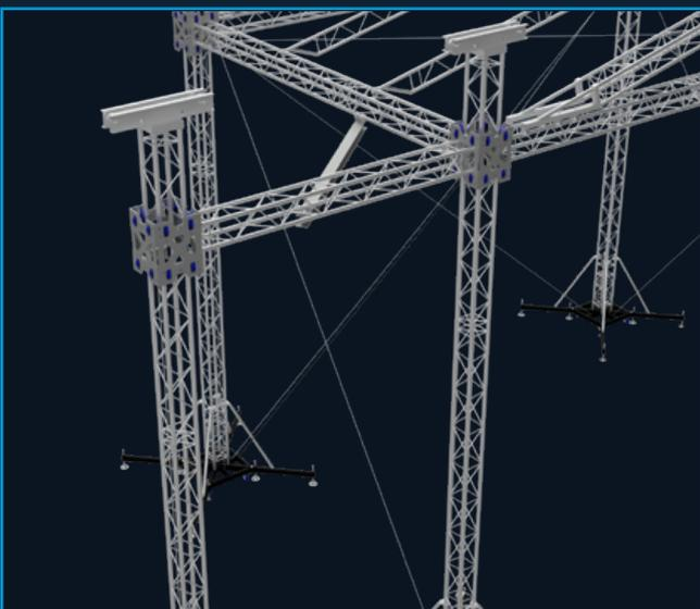
For the SDR30 roof PA Wings are available and extend the width of the SDR roof by ~3,5 meters on each side. The PA Wing itself is 3 meters in width. The maximum load is 1.000 kg CPL on each side.
