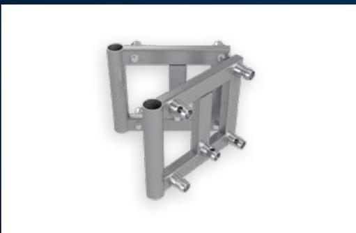
Book corners offer users increased flexibility for endless angle adjustment between 1° and 180°. The corners are designed so that a bolt must be inserted through the aluminum hinge frame to connect the female receivers or male half connectors.
