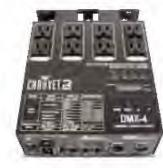
DMX-4 is a 4-channel dimmer/relay pack equiped with an automatic ON/ OFF when DMX signal is detected. It provides DMX control and/or dimming to units not equipped with DMX on their own. It is optimized for use with small LED fixtures to prevent ghosting and flickering. Each of the 4 sets of outlets (duplex) can be set to any DMX address and independently set as a dimmer or relay. Sixteen user-selectable chase patterns make programming a breeze.
