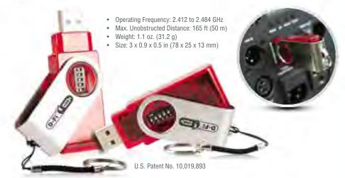
CHAUVET DJ has developed a series of fixtures that include a standard USB connection. You can now wirelessly connect to all of them using the new D-Fi USB transceiver, which eliminates the need for any DMX cables. The USB transceiver is powered directly from the fixture. Control your USB fixtures using any of our wireless controllers, or from your smartphone with the D-Fi Hub and FlareCON.
