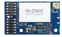
The transceiver supports our innovative Flex mode, meaning the card can be quickly and easily changed between transmitter and receiver.
