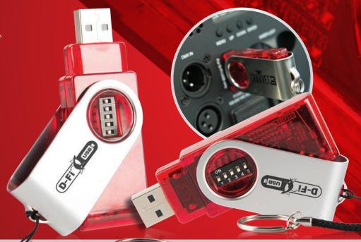
CHAUVET DJ has developed a series of fixtures that include a standard USB connection. You can now wirelessly connect to all of them using the new D-Fi USB transceiver, which eliminates the need for any DMX cables. The USB transceiver is powered directly from the fixture. Control your USB fixtures using any of our wireless controllers, or from your smartphone with the D-Fi Hub and FlareCON.
