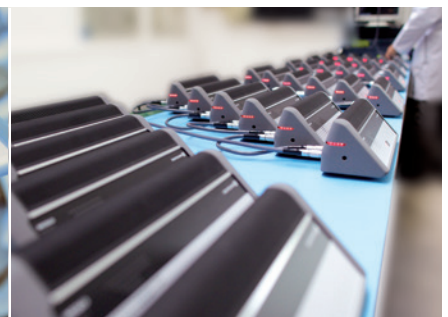
Every system undergoes a 24-hour system test
