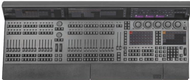
The grandMA3 full-size Control Room Version (CRV) console is the flagship of the range but supplied without the monitor wing. Designed for use in control rooms where sightlines can be challenging, the grandMA3 full-size CRV features 3 additional external monitor ports to facilitate the convenient location of external 3rd party touchscreens without compromising the grandMA3 full-size console functionality.
