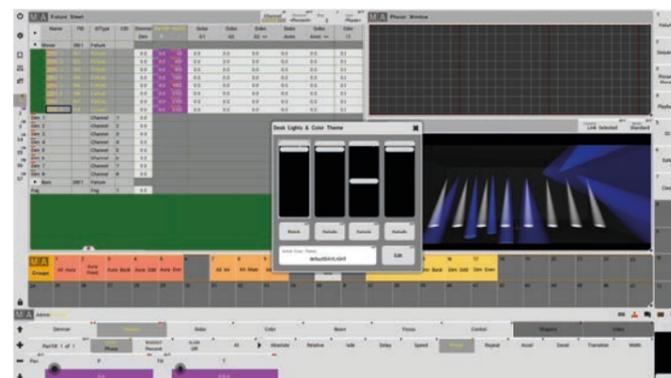
The playback options on grandMA3 allow for maximum usability of all sequences. Users can now assign any function to any action of a button, fader or encoder. From a simple GO+ functionality on a single button press, to fast-forwarding when an encoder is turned clockwise and fast-backwards when turned anti-clockwise.
