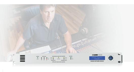
DN9650 provides a multichannel interface between AES50 networks and third party digital audio networks and point-to-point interfaces. The AES50 and third party interfaces operate in separate clock domains and are connected by a bidirectional asynchronous sample rate converter (ASRC). This unique KLARK TEKNIK technology allows the interfacing of up to 64 bidirectional channels
