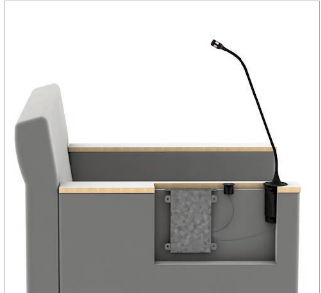
Armrest installation with a gooseneck microphone of the Classis microphone series, shockmount and button. The Orbis SU 63 system unit is mounted upright into the armrest.
