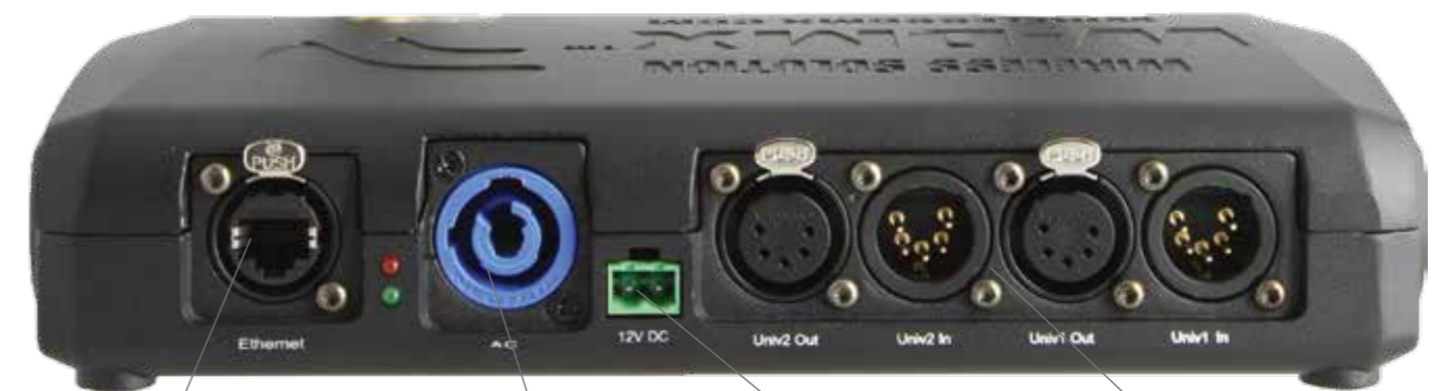
NEUTRIK ETHERCON ART-NET & S/ACN OPTIONAL PoE (POWER OVER ETHERNET) OPTIONAL NEUTRIK POWERCON 90-250V 12V PSU 3-PIN XLR AND 5-PIN XLR DEPENDING ON MODEL
