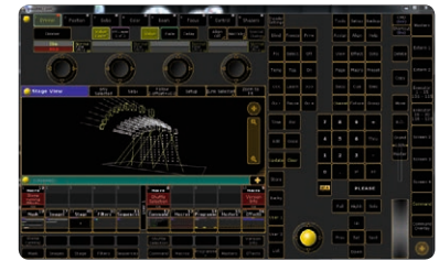
Live show controller, backup system and preprogramming Tool – grandMA2 onPC
