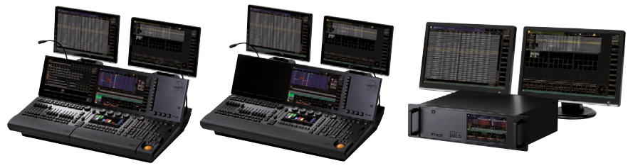
grandMA2 – Multi-User-Mode and backup solution (via 1GB/s MA-Net2)
