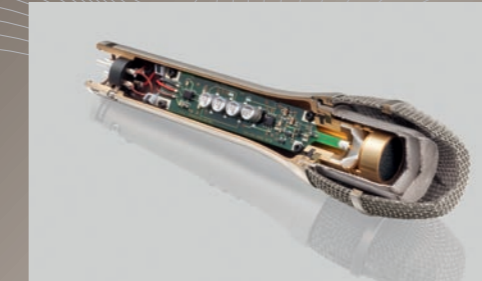
The inner-workings of the TG V96c reveal its complex design: below the exterior grill made from double-layered metal gauze, which can be easily unscrewed for cleaning, there are two further layers of metallic mesh, which serve both to protect the diaphragm and optimise the sound.
