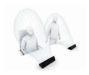
The horizontal arrangement of the microphone array results in a vertical corridor characteristic, which allows enhanced freedom of movement. Whether the speaker is sitting or standing, the volume and audio quality always remain the same. People on the left and right from the speaker are faded out.
