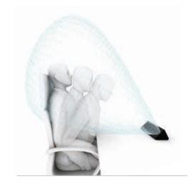
The speaker can be close to the microphone or further away. Due to the array technology, sound fluctuations are minimised by different speech distances.
