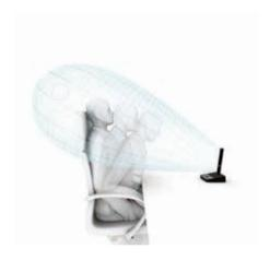
The speaker can be close to the microphone or further away. Due to the array technology sound fluctuations are minimised by different speech distances.
